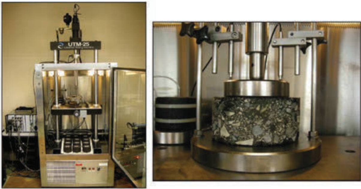
Figure 3: Universal testing machine (left) and dynamic creep test (right)
