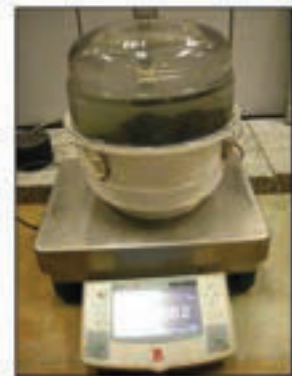
Figure 5: Uncompacted sample for G_{mm} measurement (left) and sample placed in a pycnometer (right)
