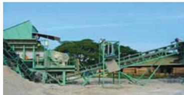
Stage 2: Ferrous metals are removed using magnetic separators.
