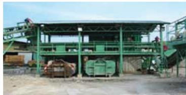
Stage 3: Foreign materials such as bricks, plastics and asphalt are screened and removed.
